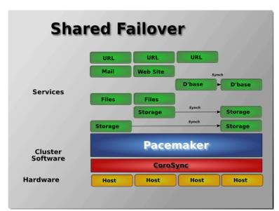
By supporting many nodes, Pacemaker can dramatically reduce hardware costs by allowing several active/passive clusters to be combined and share a common backup node Figure 1.2. Shared Failover
