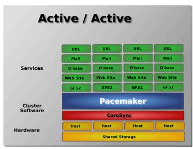
When shared storage is available, every node can potentially be used for failover. Pacemaker can even run multiple copies of services to spread out the workload.
